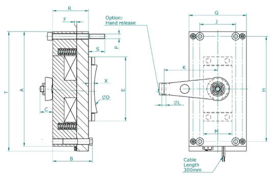
Tolerances on the supply voltage at the brake terminals =5% / -10% (NFC 79-300).
