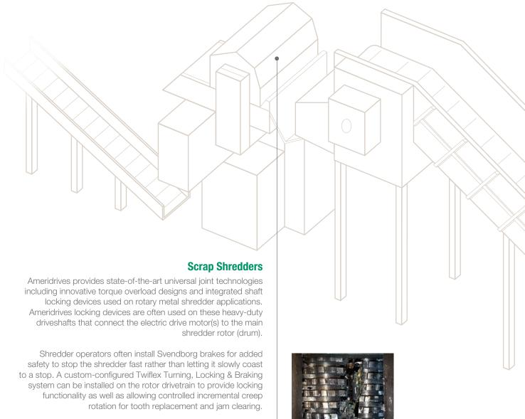
**Ameridrives** Americardan 5000 & 3000 series universal joints, Amerigear® couplings, overload devices, and Ameriloc® shaft locking devices
