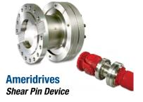
Units feature replaceable torque limiting shear pins. Pins are preset to desired torque limit. Pin count based on torque requirements.
