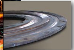
Severe damage on non-genuine copper wear plate
