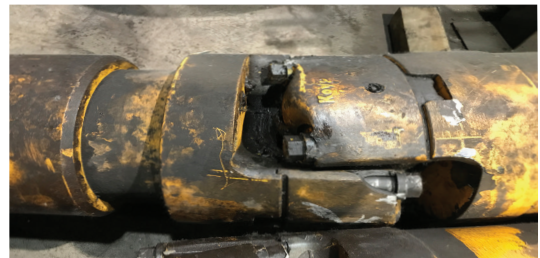
Damage due to bolts coming loose on competitor block-type U-Joint.
