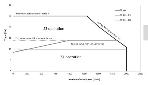
The motor is determined by the effective motor torque and the average motor speed. Both values Meff and neff must be below the S1 limit characteristic curve of the motor to be selected.
