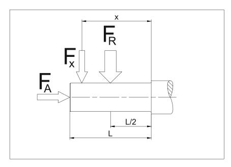
$F_{R(N, V)}$  Allowable radial force (x = I/2) according to the selection tables [N] X Distance from shaft junction to the force application point [mm]
