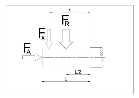
$\begin{array}{ll} F_{R(N,\,V)} & \text{Allowable radial force } (x=I/2) \text{ according to the selection tables } [N] \\ X & \text{Distance from shaft junction to the force application point } [mm] \\ F_A & \text{Axial force } [N] \end{array}$
