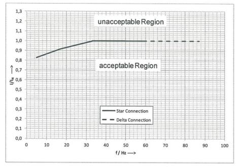
Setting parameters for the continuous current limit of the frequency converter from 5 Hz to 87 Hz
