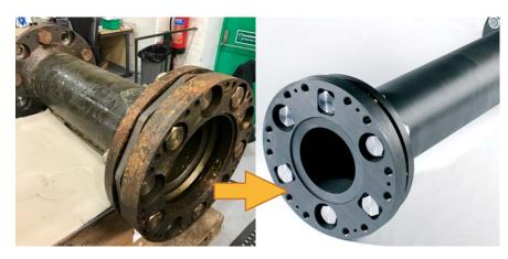
Couplings are received, inspected and rebuilt in the shortest possible time frame. We will work to accommodate your shut down schedule.
