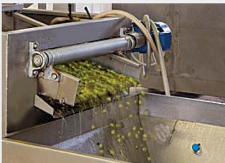
**Problem:** A large olive producer had tried various epoxy-coated speed reducers and found that they could not hold up to the acidic brine solutions and oils used on the processing lines.
