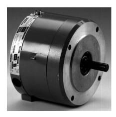
These double C-Face Brakes are direct acting with only one moving part. They are spring set and electro-magnetically released. Movement is limited to a spring loaded pressure plate. Release is instantaneous. If power fails, the brake will immediately set and hold.
