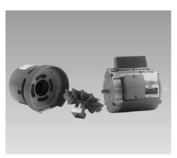
Kit includes all of the components needed for conversion of a 56C or 143-5TC frame totally enclosed fan cooled motor\* to a brakemotor. (Totally enclosed Stearns brake, replacement cast fan cover, shaft extension and fan/hub.) Mounts on fan end of motor. May be used on single or three phase motors.
