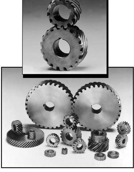
Boston helical gears are stocked both right and left hand, made with a 45° helix angle. They are designed to transmit motion and power between non-intersecting shafts which are positioned either parallel (opposing hand) or at 90° to each other (same hand). Because these gears are top-hobbed, there is extremely close concentricity between the pitch diameter and the outside diameter.
