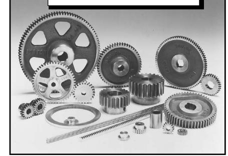
Boston spur gears are designed to transmit motion and power between parallel shafts. Configurations include spur, rack, pinion wire, stem pinions and internal gears; most with a selection of bores, keyways and set screws. Fine-pitch gears are available in plastic, brass, stainless steel and steel. Heavier pitch spurs are available in steel and cast iron. Styles include plain, web, web with lightening holes or spoked. Change gears have consecutive numbers of teeth for a variety of ratios.
