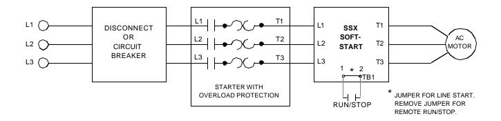
FIGURE 2-3. WIRING DIAGRAM, SSX CONTROLLER
