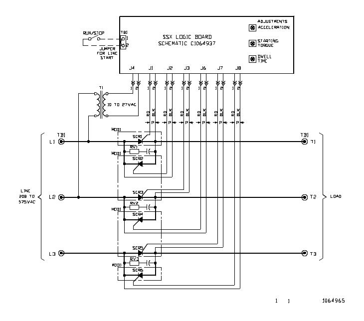
FIGURE 8-1. SCHEMATIC, MODEL SSX0076 AND SSX0310 CONTROLLERS
