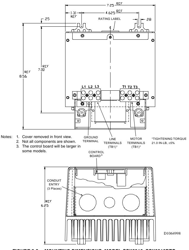
FIGURE 2-2. MOUNTING DIMENSIONS, MODEL SSX0310, SSX0310DTC, AND SSX0520DTC CONTROLLERS
