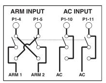
Connection for RBX Series: The customer provides interconnecting wiring.
