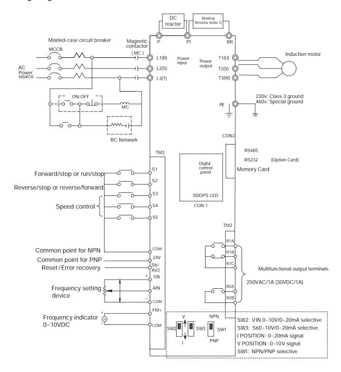
Note 1: Please refer to description of main circuit terminals (P1, BR) and specification of braking resistor for value selection. (Table 6.2 Dynamic Braking Resistor)
