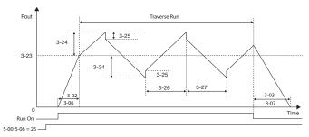
2. During traverse run, the center frequency could be controlled by the multifunction input terminals. However, the X upper deviation and Y lower deviation cannot be input at the same time. If they are inputted at the same time, the drive will maintain the original center frequency. The motion is as the graph below:
