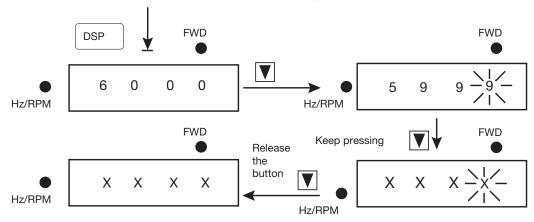
Note: XX . XX shows the present output frequency. The value ranges from 59 58 to 0 Hz, depending on the length of time the ▼ key is pressed.
