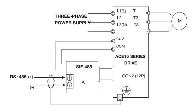
**Note:** Please put on the cover of drive to avoid the Interface Card distrubed by outside static electricity.
