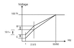
4. When the induction motor is running, there must be slip due to the load. It is necessary to boost the slip frequency to improve the regulation of the speed.
