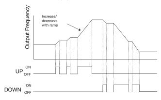
5-09=0.01 to 5.00, UP/DOWN terminal ON, that equivalent to increase/decrease the frequency of parameter 5-09. If the pressing is over 2 seconds, renew the original UP/DOWN mode. (Please refer to the following diagram.)
