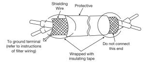
For 230V class ground 100 $\Omega$  or less; for 480V class ground 10 $\Omega$  or less.
