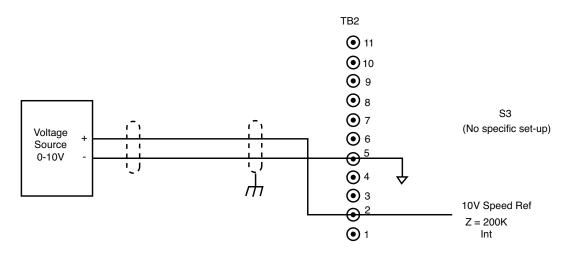
Figure 18. Signal Connection, 0-10 VDC External Speed Reference
