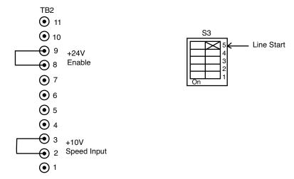
Figure 14. Signal Connection Diagram, Line Starting without a Motor Speed Potentiometer
