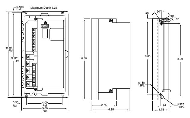
Figure 2. Controller Mounting Dimensions
