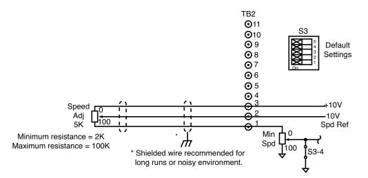
Figure 11. Signal Connection Diagram, Motor Speed Potentiometer
