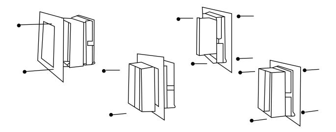
Figure 1. Base Mounted Controller Mounting Configurations
