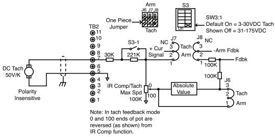
Figure 12. Signal Connection Diagram, Tachometer Feedback
