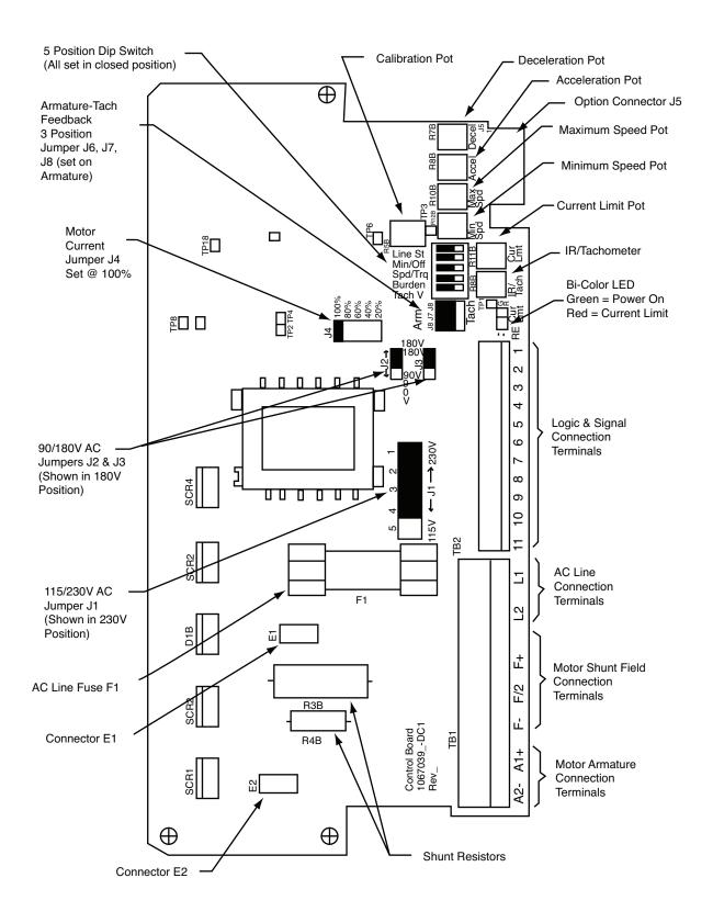
Figure 20. BETA II Control Board, 1/6 - 3 HP
