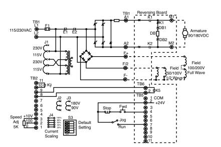
Figure 9. Logic Connection Diagram, Optional Armature Contactor Reversing Using Pushbuttons and Run-Jog Switch
