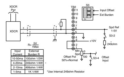
Figure 17. Signal Connection Diagram, Transducer with External Burden Resistor
