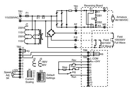
Figure 10. Logic Connection Diagram, Line Starting with Motor Speed Potentiometer
