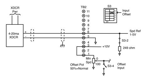
Figure 15. Signal Connection Diagram, 4-20 mA Interface
