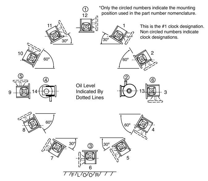
For Single Reduction Cast Iron Units Only: Refer To Lubrication & Installation Instructions Please note the clock designations (1 through 12) do not correlate with the part number nomenclature.
