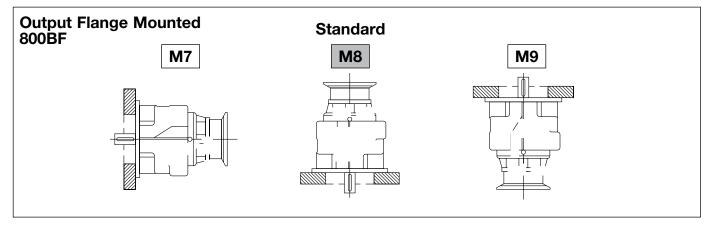
Positions M1 & M8 are standard and will be supplied with oil for this position unless otherwise specified.
