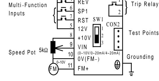
• Grounding circuitry must not be formed when grounding several controllers together.
