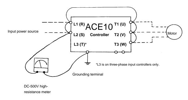
Connection for dielectric strength test
