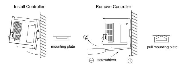
First, place the groove on the back of the controller on the upper edge of the din rail, and then push the controller down to lock up position. Finally, press the mounting plate upward into the controller.
