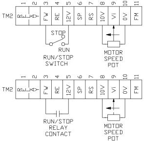
FIGURE 1. POT RUN STOP OPERATION BY SWITCH OR RELAY CONTACT WITH SPEED CONTROL BY SPEED POT OR KEYPAD
