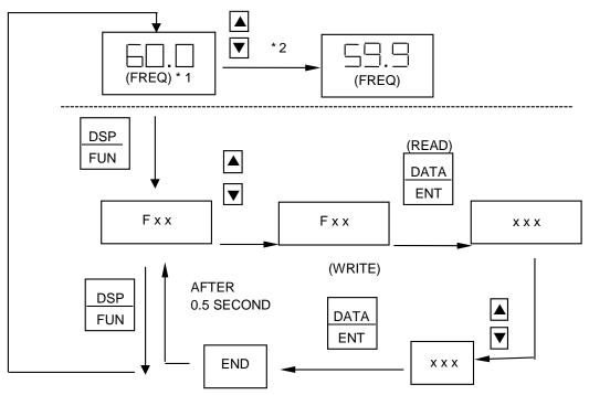
Note \*1: Displays frequency setting when stopped. Displays output frequency when running. Note \*2: The frequency setting can be modified either when stopped or when running.
