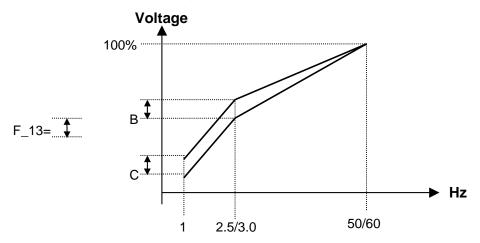
**Note**: When  $F_{13} = 0$ , the torque boost function is disabled.
