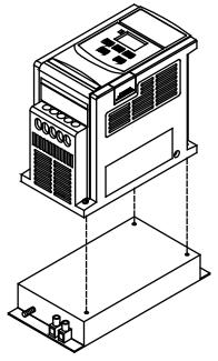
Controller with class B filter mounted.
