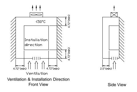
Note: Maximum temperature in the enclosure: 50°C (122°F)
