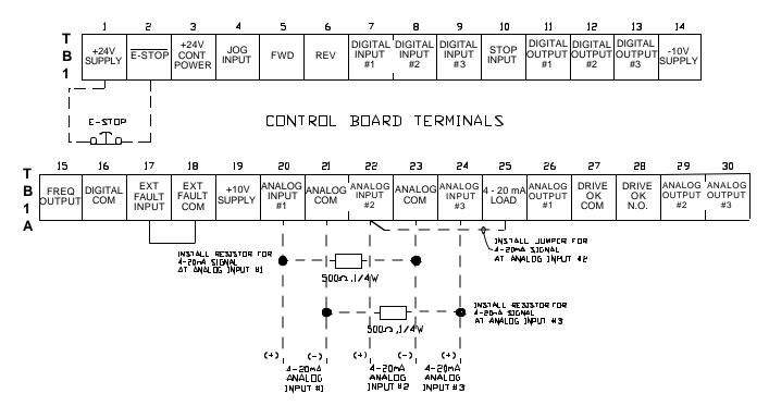
WIRING DIAGRAM, ANALOG INPUTS
