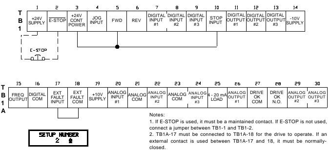
3. Use Setup #2 for Line Starting Without Auto Restart, or use Setup #3 for Line Starting With Auto Restart. See page 7-1 for more information.
