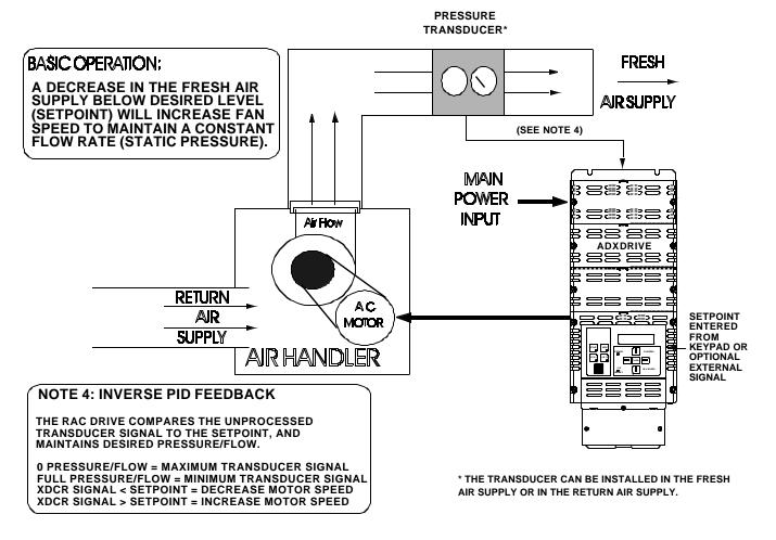
FIGURE 7-8. TYPICAL EXAMPLE OF AN AIR HANDLING APPLICATION USING INVERSE PID CONTROL (SETUP #9 OR SETUP #11)
