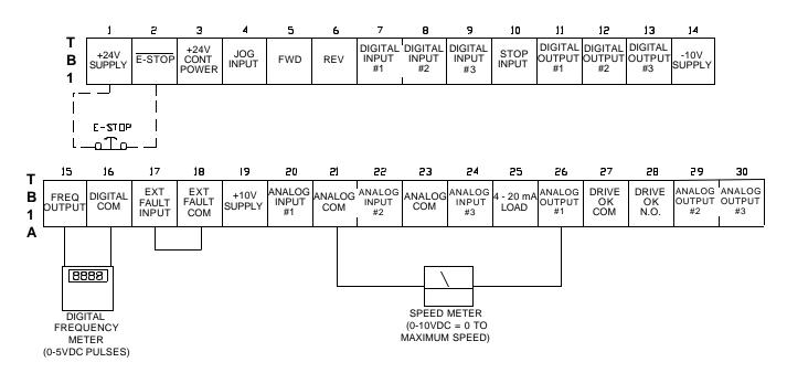
FIGURE 6 - 12. WIRING DIAGRAM, FREQUENCY & SPEED METERS - KEYPAD OR REMOTE OPERATION
