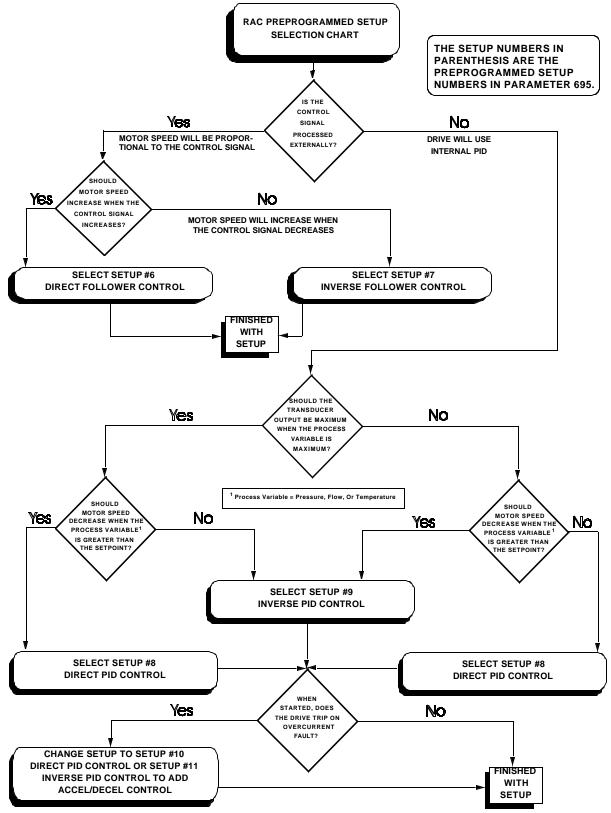
FIGURE 7-4. RAC PREPROGRAMMED SETUP SELECTION GUIDE
