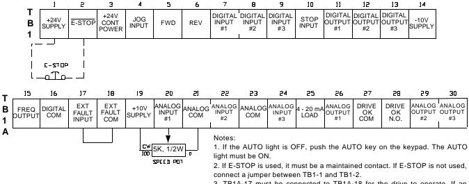
3. TB1A-17 must be connected to TB1A-18 for the drive to operate. If an external contact is used between TB1A-17 and 18, it must be normally-closed.
