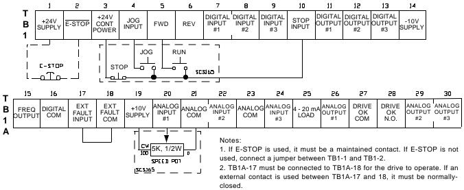
3. Set the Run Speed Source (Parameter 680) to ANALOG INPUT #1.
