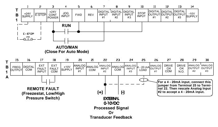
FIGURE 7-10. TYPICAL WIRING DIAGRAM FOR APPLICATIONS WITH DIRECT FOLLOWER CONTROL (SETUP #6), INVERSE FOLLOWER CONTROL (SETUP #7), DIRECT PID CONTROL (SETUP #8 OR #10), OR INVERSE PID CONTROL (SETUP #9 OR #11)
