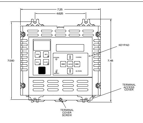
FIGURE 2-1. ADX CONTROLLER MOUNTING DIMENSIONS, 1 - 5HP, 230/460V
