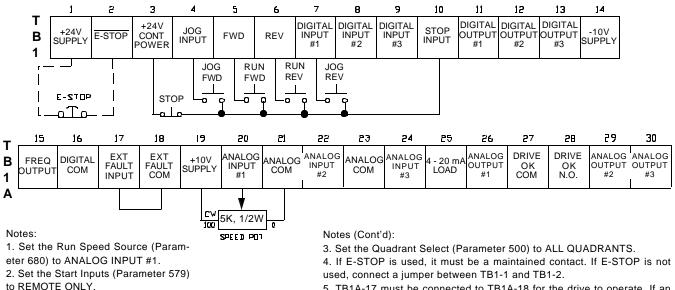
5. TB1A-17 must be connected to TB1A-18 for the drive to operate. If an external contact is used between TB1A-17 and 18, it must be normally-closed.
