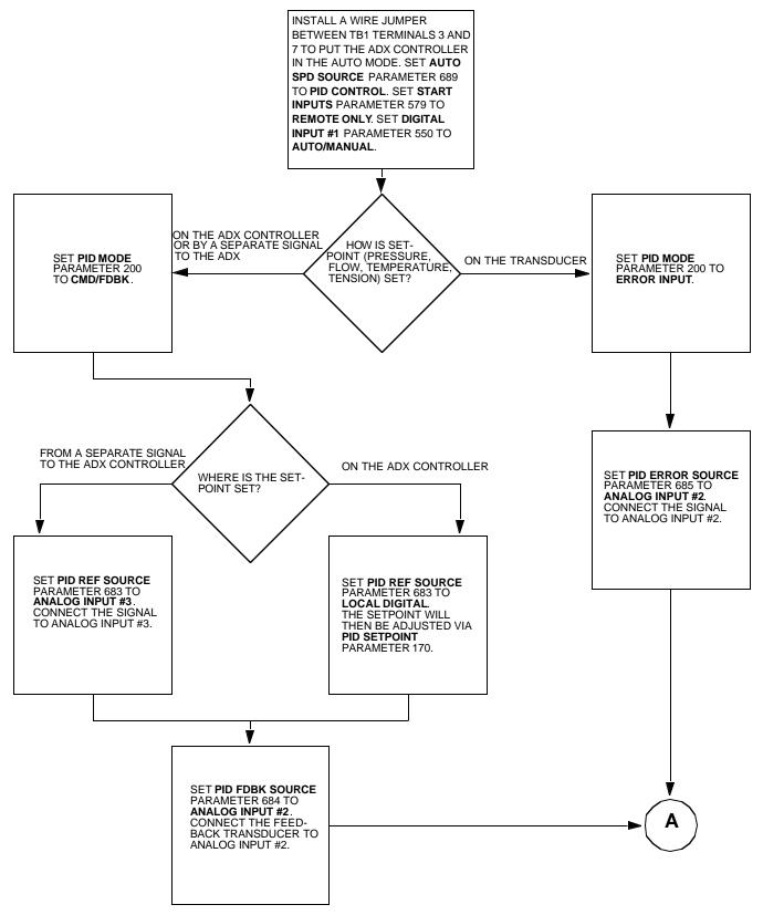
FIGURE 8 - 3. PID SET-UP FLOW CHART FOR PROCESS CONTROL (Cont'd On Next Page)
