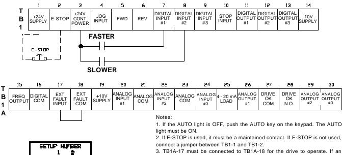
external contact is used between TB1A-17 and 18, it must be normallyclosed. 4. The preset setting for Start Inputs Parameter 579 is KEYPAD ONLY. If
