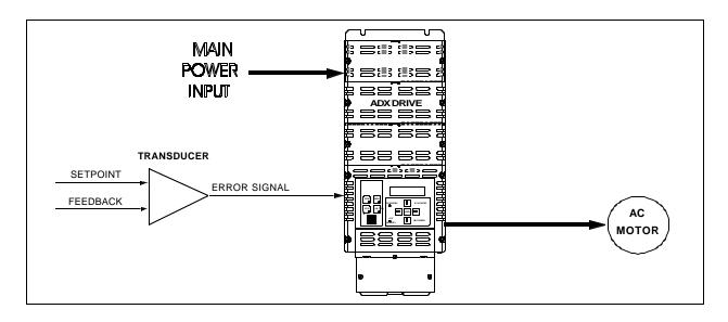
FIGURE 8 - 2. BLOCK DIAGRAM, PID ERROR INPUT MODE
