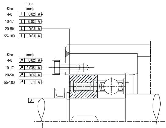
The AS clutch must be mounted adjacent to bearings to provide the concentricity and to support any axial and radial loads. Oil or grease lubrication must be provided along with seals to retain the lubricant.
