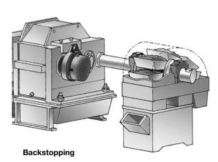
FHB backstops are mounted on the double extended input shaft of gear reducers and provide instantaneous automatic backstopping to the drive system for typically inclined conveyors and bucket elevator applications.
