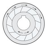
In this type of application, reciprocating motion applied to the driving race is transformed into intermittent motion in only one direction at the driven race. For example, if a pinion is connected to the driving race, a rack meshing with the pinion can give reciprocating motion to the driving race. The clutch will then advance or "index" the work (driven race) on each forward stroke of the rack, but will not return or back-up on the return stroke of the rack.
