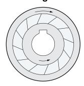
This class of applications is typified by standby and compound drives. For example, a steam turbine and a standby electric motor may be connected to a single driven shaft through overrunning clutches. The shaft can then be driven by either the turbine or the motor or both with no further modification of the installation. The turbine drive clutch automatically engages when the turbine starts to drive, but automatically overruns when the load is transferred to the electric motor.
