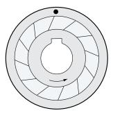
In backstopping or holdback\* applications, one race is always fixed to a stationary ground member. The function of the clutch is to permit rotation of the mechanism, connected to the other race, in one direction only, and to prevent any rotation in the reverse direction at all times. Although the clutch normally overruns most of the time, it is referred to as a holdback or backstop in conveyors, gear reducers and similar equipment because its function is to prevent reverse rotation.
