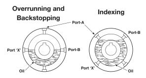
Note: Models EP-300 through -600 do not have Port 'X'. Position as shown without Port 'X'
