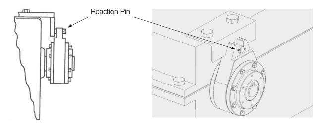
The Model FHB can be axially restrained by a cotter pin in the reaction pin
