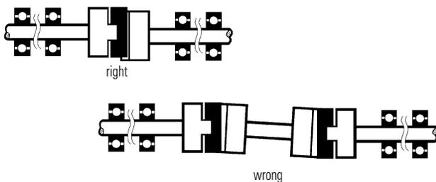
Note: It is important that installed couplings are not end-loaded. To help avoid this, thro' bored hubs are recommended for shafts which have fixed axial locations such as face-mounted motors.
