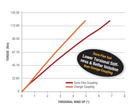
The Dura-Flex elastomer coupling has been proven to optimize torque transmission, while minimizing parallel, angular, and axial
