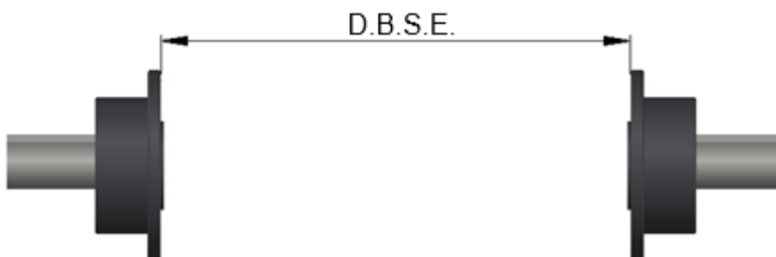
DBSE distance is the distance between the hub faces
