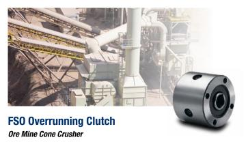
A mine equipment manufacturer required a reliable overrunning clutch for use on a cone crusher. Ore is crushed between an eccentrically rotating cone mantle and a concave bowl liner. The clutch prevents the mantle head from rotating in the reverse direction from the design parameters.
