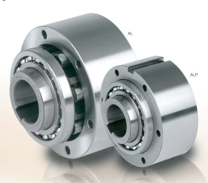
ypes AL, ALP are roller type freewheels. These units are part of the Stieber modular system. They are bearing supported, using two 160.. series bearings, and require oil lubrication. These units may be used in designs providing oil lubrication and sealing as on the example overleaf.
