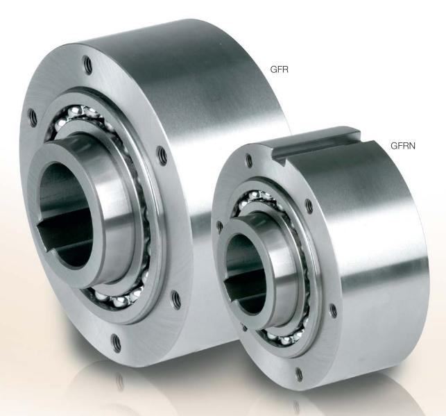
ypes GFR, GFRN are roller type freewheels. These units are part of the Stieber modular system. They are bearing supported, using two 160.. series bearings, and require oil lubrication. These units may be used in designs providing oil lubrication and sealing as on the example overleaf. The bearings must not be axially stressed.
