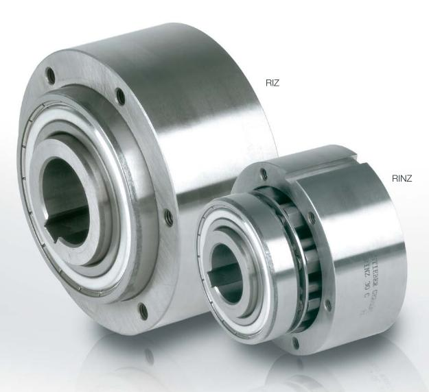
ypes RIZ, RINZ are centrifugal lift off sprag type freewheels with the inner race rotating. Suitable for backstop, or overrunning clutch applications. Only the inner race is designed for freewheeling.
