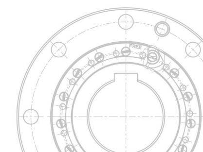
The RDBK is a centrifugal lift-off sprag type backstop which is designed for use on the high speed or intermediate shaft. With an internal torque limiter, the RDBK is designed for the use on large inclined conveyors, where the release function or load sharing is required. The RDBK also protects the conveyor belt system by cutting the peak loads.
