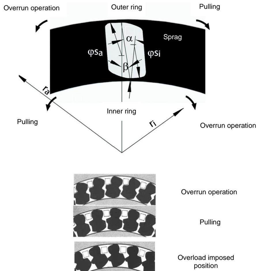
Fig. 2 Pulling/overrun operation
