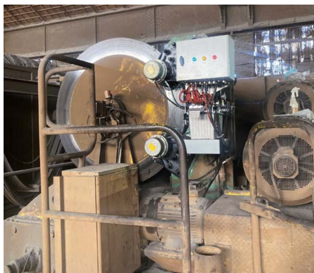
Revamping / 175T TAIM Industeel Le Creusot crane with SIMAN modules (K-SI electrical units)
