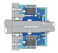
**Stromag KMK** for use in gearboxes (wet operation) with optional disc oil flushing. Hydraulic and cooling oil supplied via the transmission shaft.
