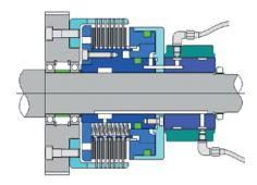
**Stromag KMK** for use in gearboxes (wet operation) with optional disc oil flushing. Hydraulic and cooling oil supplied via integrated radial oil supply (KRE).
