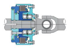
**Stromag KMK** as a shaft-cardan shaft connection for use outside gearboxes (dry operation). Hydraulic oil supplied axially through the shaft. Available as a completely assembled and bearing supported unit.
