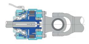
**Stromag KHR** as a complete unit for preassembly with supported external body as a shaft-shaft connection.
