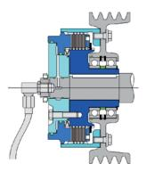
**Stromag KMK** as a shaft-pulley connection for use outside gearboxes (dry operation). Hydraulic oil can be supplied axially through the shaft. Available as a completely assembled and bearing supported unit.
