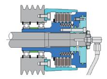
**Stromag KUK** as a shaft-pulley connection for use outside gearboxes (dry operation). Hydraulic oil supplied axially through the shaft. Available as a completely assembled and bearing supported unit.
