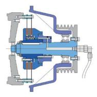
**Stromag KHM** for engine mounting. Backlash-free power transmission via diaphragm guided pistons and friction linings. Drag torque free when open. Connection for SAE flywheels. Housings for SAE sizes 1 to 4 possible.
