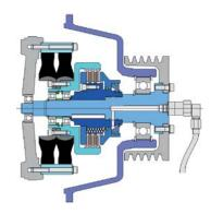
**Stromag KHA** with flexible Periflex<sup>®</sup> VN couplings for drives particularly subject to torsional vibrations. Connection for SAE flywheels. Housings for SAE sizes 1 to 4 possible.
