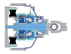
**Stromag KHR** as a "Two in One" combination in SAE housing on diesel engine with direct flange-mounted cardan shaft.
