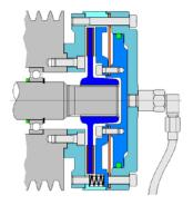
**Stromag KHM** as a shaft-pulley connection. Backlash-free power transmission on pulley side through external body and piston with diaphragm guidance. Friction lining carrier on shaft side with low wearing, wide sliding gear.
