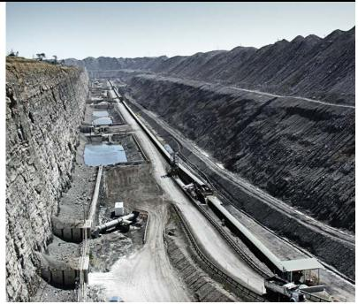
Conveyors are efficient in industrial mines and metallurgical plants. But like other heavy equipment, they pose hazards to employees and to the safety of the equipment, as the operation is mostly unmanned due to its distance, terrain and profile. Therefore, it is imperative to develop an intelligent soft braking system to address the starting and stopping requirements under various load conditions.
