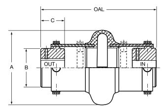
Shaft Spacing from 6.35 mm up to the MAX DBSE can be accommodated by positioning hubs IN or OUT or by using various existing hole patterns. OAL — Over All Length does Not include bolt heads.
