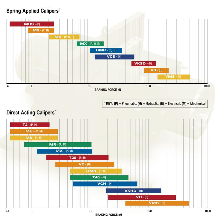
\*It should be noted that the braking forces shown are for a single caliper only and multiple calipers may often be used on a disc, with available space being the typical limitation.
