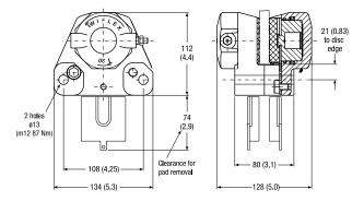
The standard Twiflex T20 disc brake is a side-mounted, split caliper design suitable for use with a minimum disc thickness of 12.7mm. Thicker discs may be accommodated by inserting an appropriate size spacer between the two caliper halves. If the disc thickness is greater than 20mm the spacer may also be configured as a central mounting plate. Optionally, the caliper may be supplied in a modified form for use with a minimum disc thickness of 8mm. Minimum disc diameter is 300mm.
