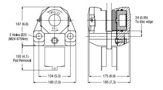
The Twiflex T40 disc brake caliper is split caliper design suitable for use with a minimum disc thickness of 20mm. The modules are mounted each side of a central mounting plate of the same thickness as the brake disc. Minimum disc diameter is 300mm.
