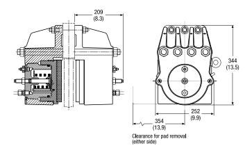
The Twiflex VKHD disc brake caliper is comprised of two halves, or hydraulic modules, and is suitable for use with a minimum disc thickness of 20mm. The modules are mounted each side of a central mounting plate 12mm thicker than the brake disc. Minimum disc diameter is 1000mm.
