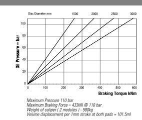
The ratings shown on the graph are based on fully bedded in and conditioned brake pads with a nominal friction coefficient  $\mu = 0.4$ . Twiflex disc brakes must be used with Twiflex asbestos free brake pads.
