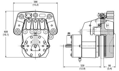
The Twiflex VKSD-FL disc brake caliper comprises a single spring module forming the 'active' side of this floating unit and is available for use where space is limited or to accommodate axial disc float of ±6mm.
