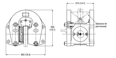
Disc Diameter mm 1200 1600 2000 2500 140 120 100 bar 0il Pressure – 800 60 40 20 ٥ 50 100 150 200 250 300 350 Braking Torque kNm Maximum Pressure 140 bar Maximum Braking Force = 285kN @ 140 bar Weight of caliper - 287kg Volume displacement per 1mm stroke at both pads = 51.7ml
