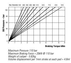
Normally one or two calipers are used per disc, but the number may be increased depending on disc size. The brakes may be positioned at any angle around the periphery of the disc. A range of brake discs is available from Twiflex (see Disc and Hub Assemblies).
