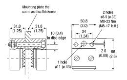
The Twiflex T2 disc brake caliper is split caliper design suitable for use with a minimum disc thickness of 5mm. The modules are mounted each side of a central mounting plate of the same thickness as the brake disc. Minimum disc diameter is 120mm. Alternatively, the brake may be side-mounted with a spacer equal to the disc thickness between the two halves.
