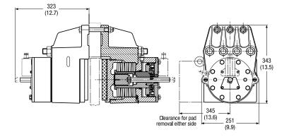
The Twiflex VKSD disc brake caliper is comprised of two halves, or spring modules, and is suitable for use with a minimum disc thickness of 20mm. The modules are mounted each side of a central mounting plate 12mm thicker than the brake disc. Minimum disc diameter is 1000mm.
