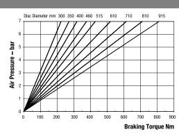
Maximum Pressure 7 bar Maximum Braking Force = 1.9kN @ 7 bar Weight of caliper and thruster - 7.3kg Weight of thruster only - 0.3kg Volume displacement of thruster at full stroke = 64ml
