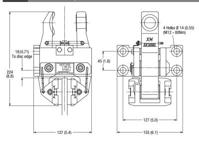
MXA Pneumatically Applied – Spring Released
