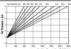
Braking Torque Nm (Full Rate)
