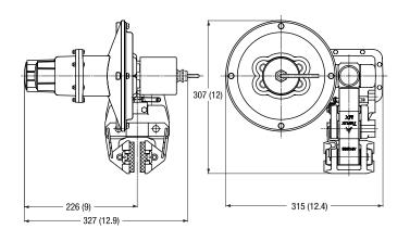
Maximum Braking Force = 6kN Weight of caliper and actuator - 15.7kg
