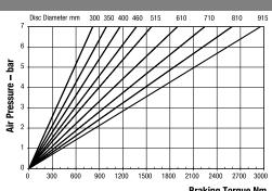
Maximum Pressure 7 bar Maximum Braking Force = 6.9kN @ 7 bar Weight of caliper and thruster - 8.32kg **Braking Torque Nm** Weight of thruster only - 1.32kg Volume displacement of thruster at full stroke = 300ml
