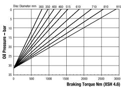
Minimum Pressure for full retraction: 40 bar Maximum Braking Force XSH 4.6: 6.8kN Weight of caliper and thruster - 11kg
