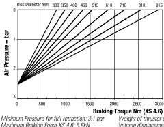
Maximum Braking Force XS 4.6: 6.8kN Weight of caliper and thruster - 11.5kg Weight of thruster only - 4.5kg Volume displacement of thruster at full retraction = 1.19 /
