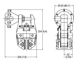
MXE Pneumatically Applied – Spring Released
