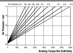
Minimum Pressure for full retraction: 50 bar Maximum Braking Force full rate: 6.4kN Weight of caliper and thruster - 11kg Weight of thruster only - 4.0kg Volume displacement of thruster at 4mm retraction = 5ml
