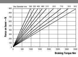
Weight of caliper and lever assembly - 8.4kg Weight of lever assembly only - 1.4kg Maximum Braking Force = 8.3kN @ 0.9kN force on lever
