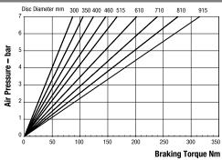
Maximum Pressure 7 bar Maximum Braking Force = 0.74kN @ 7 bar Weight of caliper and thruster - 7.34kg Weight of thruster only - 0.34kg Volume displacement of thruster at full stroke = 25ml
