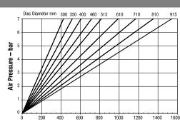
Maximum Pressure 7 bar Maximum Braking Force = 3.6kN @ 7 bar Weight of caliper and thruster - 8.15kg
