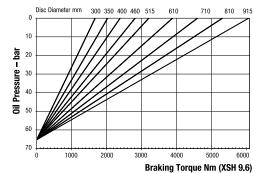
Minimum Pressure for full retraction: 82 bar Maximum Braking Force XSH 9.6: 14.3kN Weight of caliper and thruster - 11.6kg
