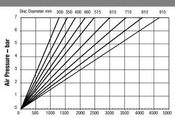
Maximum Pressure 7 bar Maximum Braking Force = 11kN @ 7 bar Weight of caliper and thruster - 9.06kg
