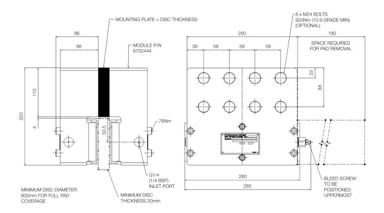
Maximum braking force = 136 kN at 150 bar (normal maximum working pressure) The ratings shown on the graph below are based on fully bedded and conditioned brake pads with nominal friction coefficient  $\mu$  = 0.4 (see Twiflex Publication P1164 for more information on typical friction coefficients). For general bedding in and conditioning procedures refer to Twiflex Publication M1060.
