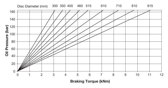
The ratings shown on the above graph are based on fully bedded and conditioned brake pads with nominal friction coefficient  $\mu$ =0.4. For bedding-in and conditioning procedures see Publication M1060.
