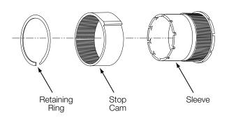
To adjust the stop collar output orientation:
