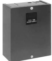
The TCS-168 power supply is designed to provide the correct power input to the TCS-310 Dancer Splicer Control. Its switch selectable input allows the user to adapt to 120 or 240 VAC. It has dual voltage circuits to provide low voltage power and anti-residual output as well as power to operate two brakes. The TCS-168 is available with an open frame for control panel mounting.
