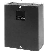
The TCS-167 power supply is designed to provide the correct power input to TCS-210 and TCS-220 tension controls. Its switch selectable input allows the user to adapt to 120 or 240 VAC. It has dual voltage circuits to provide low voltage power and anti-residual output as well as power to operate a brake. The TCS-167 is available with an open frame for control panel mounting.
