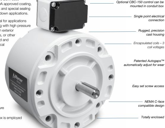
One piece, C-face package completely assembled and factory aligned. Mates easily with standard motors and reducers. Foot mounted package also available. Easy-to-install and no maintenance required.
