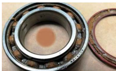
Typical example of internal bearing corrosion resulting from water ingress.
