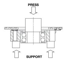
**AWARNING** Support the clutch only in the area shown and only press on the end of the mounting sleeve to prevent bearing damage.
