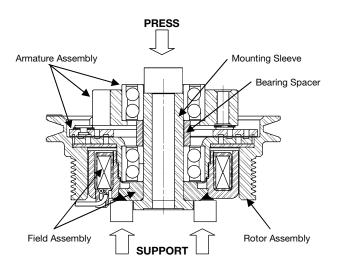
To disassemble the armature assembly, support the armature assembly on the fan spacer mounting surface with the bearing not supported. Press on the inner race of the bearing to remove the bearing. Note: Removing the bearing in this manner will cross load the bearing and the bearing can not be reused.
