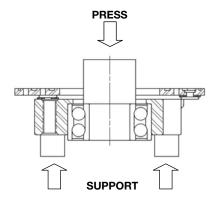
**AWARNING** Support the clutch only in the area shown and only press on the end of the mounting sleeve to prevent bearing damage.
