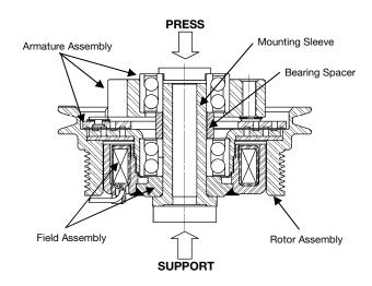
AWARNING Support the clutch on the flanged end of the mounting sleeve and only press on the inner race of the bearing to prevent bearing damage. DO NOT press on the outer bearing race!
