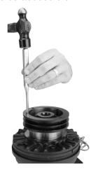
Note: For high cycle rate applications with potential pulley misalignment, apply Loctite to the I.D. of the pulley to eliminate the possibility of keyway wear.
