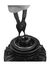
▲CAUTION When installing this or other retaining rings, be sure to hold the ring with one hand so it will not spring away should the pliers lose their grip on the ring. Always wear safety glasses when installing or removing retaining rings.
