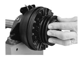
7. Tighten the hub setscrews into the shaft to the appropriate torque for your size unit:
