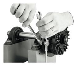
6. Tighten the set screws located in the hub to the appropriate torque for your size unit:
