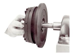
5. Install the optional Warner Electric torque arm or the customer furnished pin. The arm must be strong enough to withstand the brake's full torque capacity, and should be affixed to the machine frame, and to the brake tangent to its circumference in the notched attachment point on the back plate. It must also be flexible enough to compensate normal shaft and bearing runout without causing binding or side loading to the brake.
