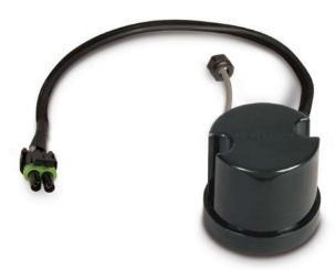
The PQS is a bi-directional current limit control. The control monitors current during actuator motion and quickly stops the actuator if an object gets in the way or at the end of stroke. The actuator will remain off until power is reapplied. The current limit setting is adjustable with two potentiometers that are accessible through two plugged holes on the side of the housing.
